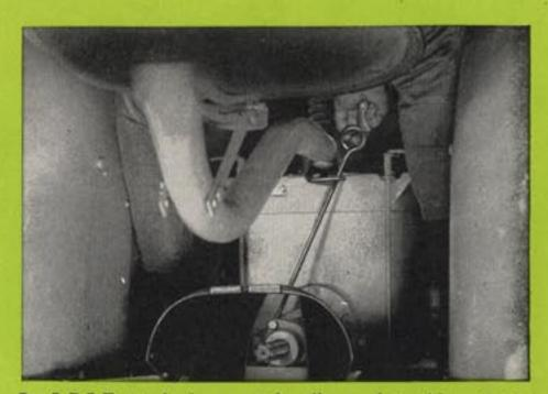
An A.S.A.E. standard power take-off, complete with protective shield, is available for use with sprayers and dusters or any other tractor-driven equipment which an orchard or grove owner might use with his tractor. As shown, the power take-off is engaged and disengaged by means of a push-pull control rod conveniently operated from the driver's seat.
