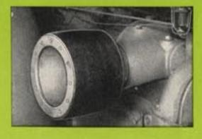
Rockwood belt pulleys are available for the O-4 and O-6 tractors. These pulleys assure a satisfactory drive with a minimum of slippage.
