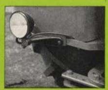
Single front and rear electric lights as shown are available as extra equipment. With strong, steady electric light the tractor can be operated day and night in rush seasons or when unfavorable weather has delayed operations past their normal time. Almost indispensable, too, for moving on the highway at night.
