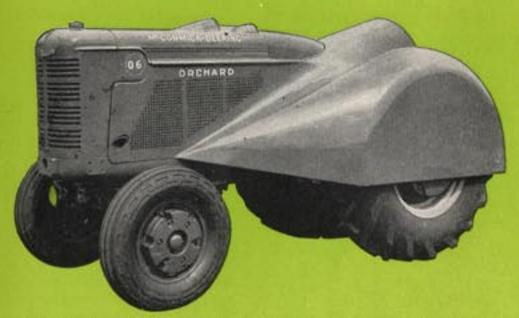
Wheel weights, both front and rear, are available in various combinations to suit the requirements or preferences of owners. (Wheel weights are not needed on solid front wheels.) The steering wheel cowl, quickly detachable when not required, is also supplied only on special order. Electric light shown is also special equipment.
