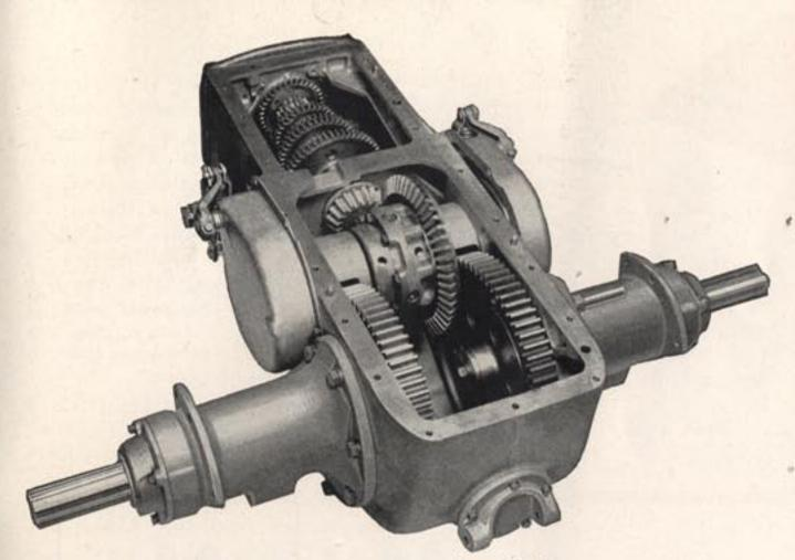
Here you get an inside view of the quiet-running, long-life, fivespeed transmission and final drive in the O-4 and O-6 tractors another good example of McCormick-Deering high-quality design and construction. Gears and pinions, large and small, are drop-forged of alloy steel, precision-machined, carburized, and heat-treated to leave them extremely hard on the contact surfaces and relatively soft in the center to absorb sudden stresses. Gear
