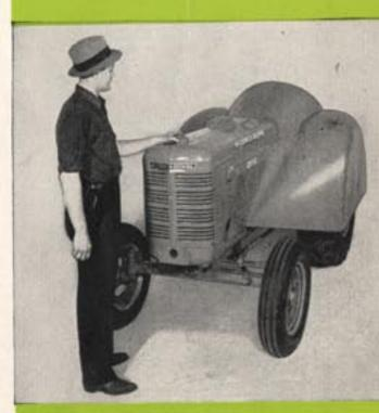
The low overall height of the McCormick-Deering Orchard and Grove tractors is readily apparent in this illustration (see specifications for height).
