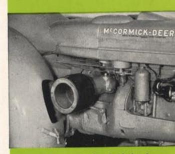
In this O-4 view the hood side has been removed to show the belt pulley (special equipment) in position for operation. Ample clearance around the pulley and a straight view along the belt from the seat make it easy to put the belt on, line it up, and tighten it.
