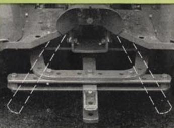
(Above) The swinging drawbar regularly supplied with "O" tractors is popular in orchard and grove work, where short turns with disk harrow and other loads are necessitated by closely planted trees.
