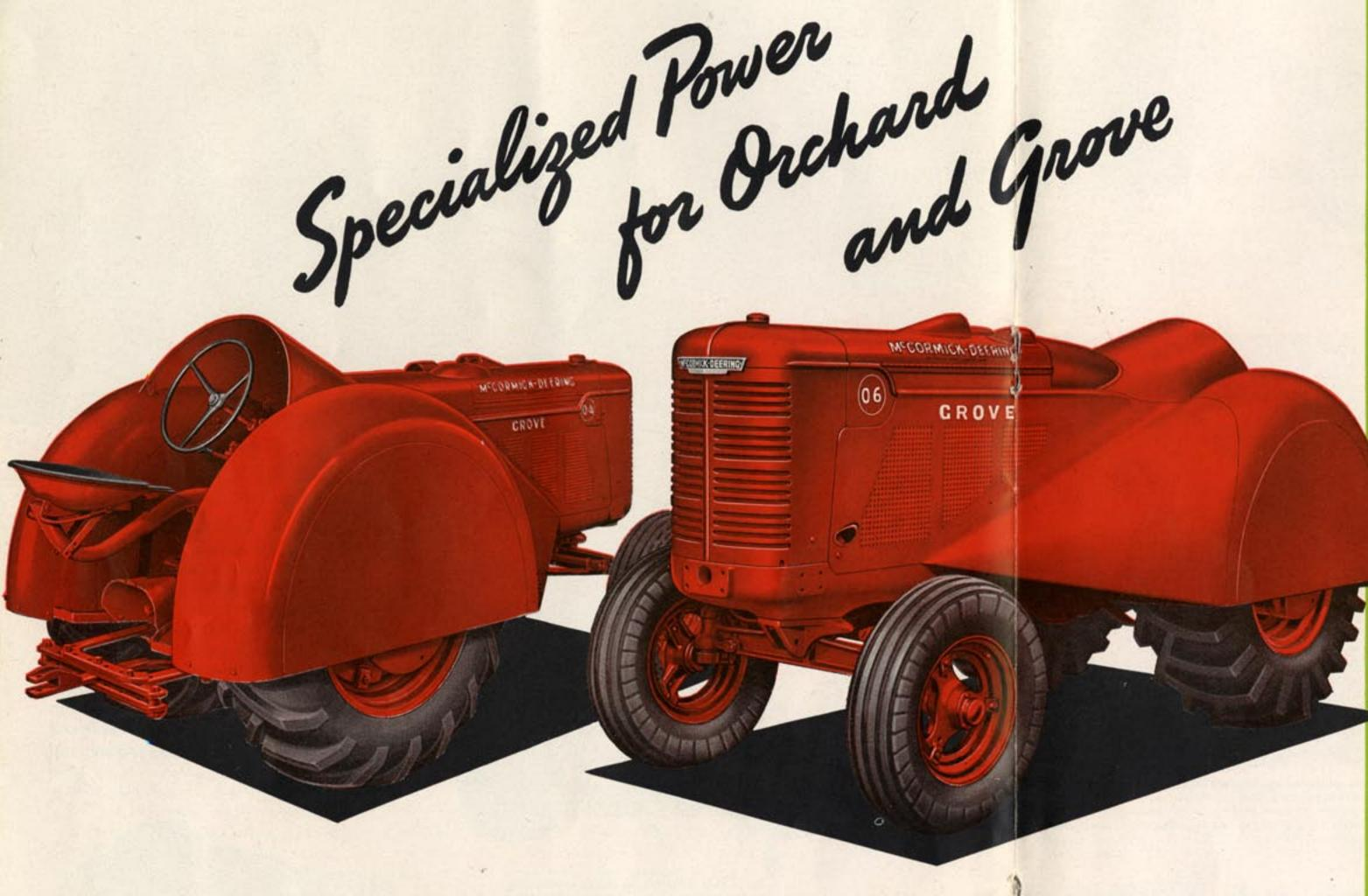
THE above illustration will give you an idea of the relative size of the O-4 and O-6 tractors. Compare these dimensions. The height of the O-4 at the radiator is 53% inches and the wheelbase is 66½ inches. For the O-6 the figures are 605% and 76 inches.
