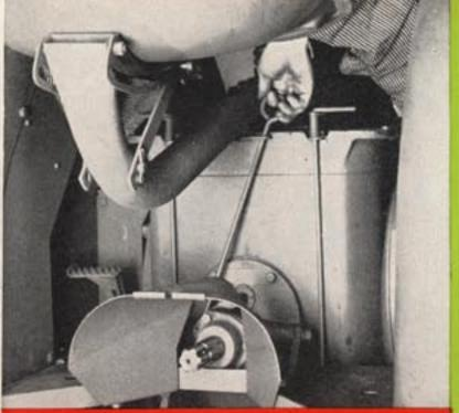
The power take-off is engaged and disengaged from the seat in the same manner as gears are shifted. Pull up to engage; down to disengage.
