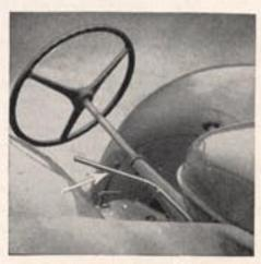
The arrow points to the variable speed governor control lever by means of which the operator can instantly obtain any desired engine speed in the full-load governed speed range. (See page 14.)
