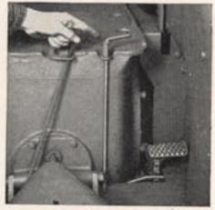
With this handy brake locking device (one for each brake) the brake can be set (note ratchet on the brake pedal) to hold the tractor stationary. Pressure on the pedal releases it automatically.
