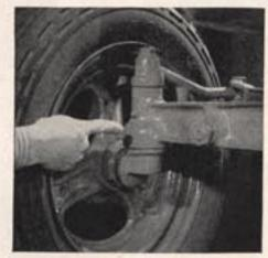
There is no "drag" in the worm and gear steering mechanism of these tractors. Ball bearings in the steering shaft housing and the forged steel steering knuckles give "finger-tip"
